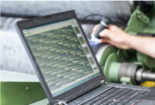
Search for damages to the wire on a roller
