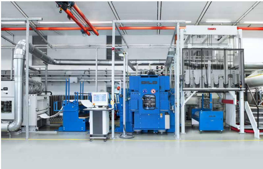
The staple fiber needle punch line at the Competence Center Felting
